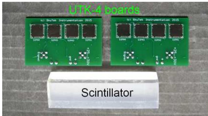
*Figure 2: Two UTK-4 boards and the piece of plastic scintillator.*
