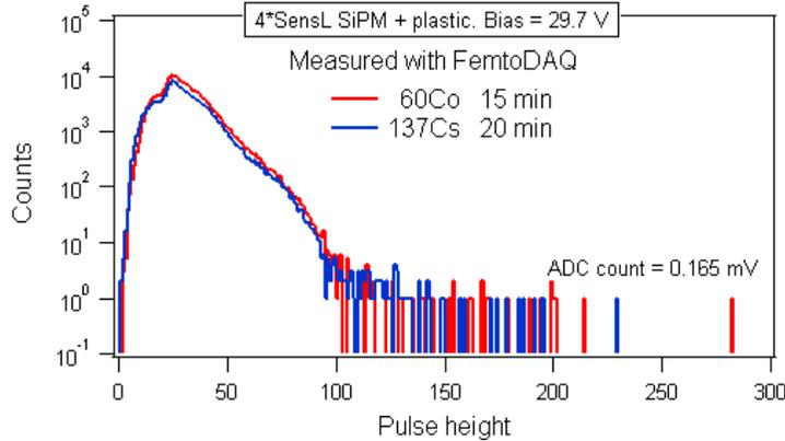
Figure 7: Pulse height distributions measured with trace amounts of rare isotopes placed on top of the detector assembly.
