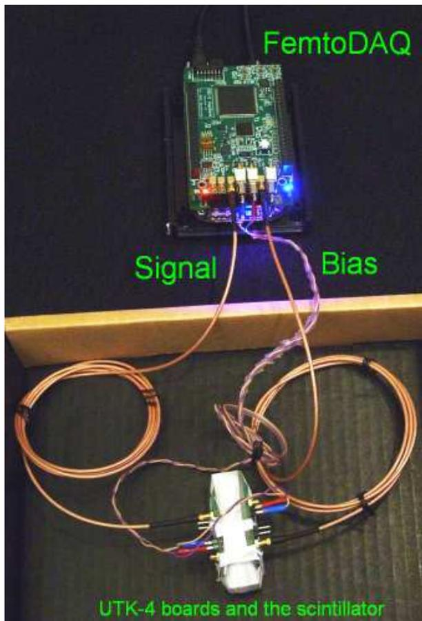
Figure 3: The scintillator assembly connected to FemtoDAQ.
